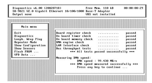
Figure 6. Typical screen display after a successful test
